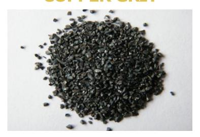
Copper grit is an abrasive sand blasting material, made of granulated slag obtained during copper melting. It is characterized by high strength and abrasiveness. The granules are sharp and curly. Sanding is achieved with a uniformly rough and sharp surface. One of the main advantages of this abrasive is the absence of dust, high strength and flexibility. Suitable for indoor use. A large specific gravity of 1.8 kg / dm3 provides a high kinetic energy of the grain when striking the surface.
